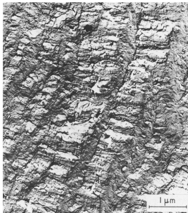
Figure 7 Transmission electron micrograph of a replica of another part of the fracture surface of the sample shown in Figure 6. Magnification 15 000 X
