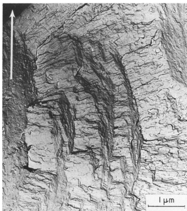
Figure 6 Electron micrograph of a replica of a fracture surface of nylon-6 crystallized at 295°C for 48 h, under pressure 6.5 kbar. The arrow shows the growth direction. Magnification 15 000 X
